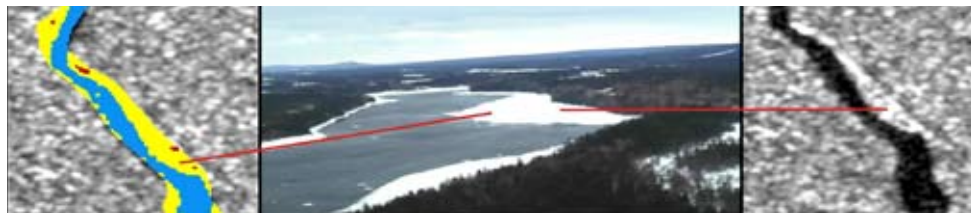
Satellite monitoring of the Exploits River is used to identify build-up of ice that may result in ice-jam flooding.
